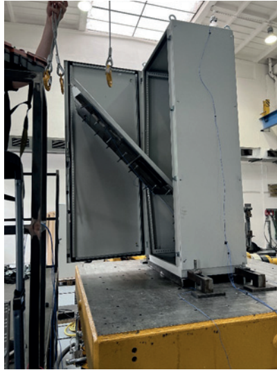
Seismic fragility testing of a newly developed modular I&C (Instrumentation and Control) cabinet for next-generation nuclear power plants. The cabinet failed during a simulation of an earthquake with a magnitude corresponding to a 100,000-year recurrence interval (by courtesy of Rizzo Associates Czech)
